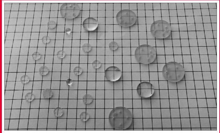
*E* lectro-Glass Products has perfected a process whereby borosilicate glasses for kovar sealing may now be offered to our customers in a clear preform. Tests show that such preforms reach 99.56% of theoretical density, thus allowing the internal seal area to be easily inspected visually.
