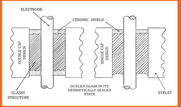
Electro-Glass Products offers a Duplex Glass preform designed to control meniscus climb and meets the requirements of MIL-STD-883C, Methods 1004, 1008-1011, 1014, 1018, 2007 & 2009.
